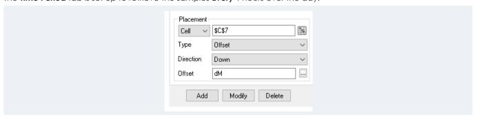
For this connection, the **Placement** is set to Offset, Down the column starting at \$C\$7 based on the day of the month (dM).
