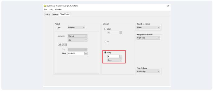
The **Time Period** tab is set up to retrieve the samples **Every** 4 hours over the day.
