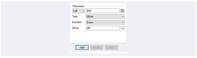
For this connection, the **Placement** is set to *Offset*, *Down* the column starting at \$1\$7 based on the day of the month (dM).
