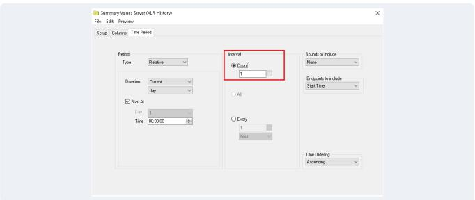
The **Time Period** tab is set up to retrieve a single row of calculations over the day.
