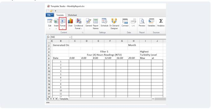
In the Template Design Studio, the template is laid out with a row for every day of the month (31 rows for worst case), columns for the 4-hour readings and columns for the maximum turbidity and the time that occurred.
