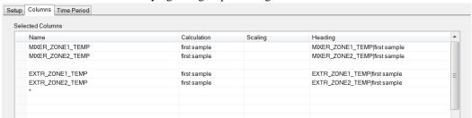
Notice an empty row is left between the *Mixer* and *Extruder* items. This is to accommodate the formula in the *E* column of the worksheet. Also notice the \* in the last column. This is configured to accommodate the formula in the *H* column of the worksheet.
