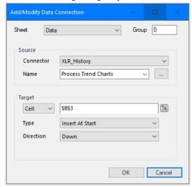
The **Sheet** indicates which worksheet the connection applies to. By selecting **Any Sheet**, the connection is applied to all worksheets. The **Any Sheet** setting is typically used in cases where multiple worksheets use the same connection. When a template update occurs involving a worksheet, only the connections with Scope set to the worksheet or **Any Sheet** are updated.
