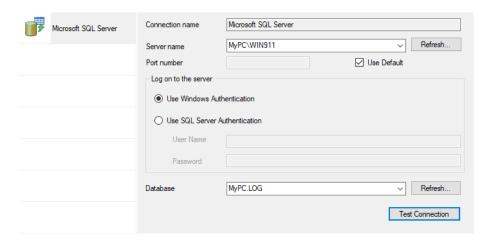
By default, the **Server name** is configured to the *WIN911* instance on the local machine, using **Windows Authentication** to the *LOG* database named after the local machine.
