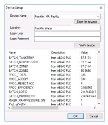
To set up a device, click **Scan for devices**. This returns a list of the Flexy devices associated with the Talk2M account specified in the **Talk2M** tab.
