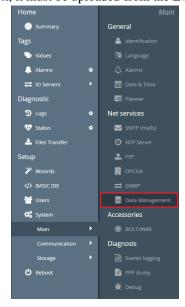
This is configured from the Ewon configuration web page by selecting **Setup**, **System**, **Main**, **Net Services**, **Data Management**.
