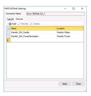
This tab is used to associate one or more Ewon Flexy devices with the Data Connector. Click **Add** to open **Device Setup**.
