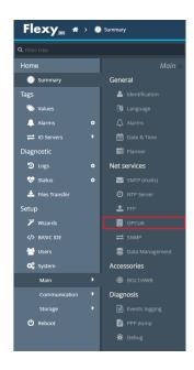
For real-time data access, enable **OPCUA** from **Setup**, **System**, **Main** in the web interface of the Ewon device.
