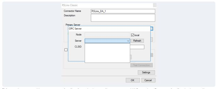
This can be caused by a communication issue between the server and XLReporter. Communication between the OPC server and an OPC client must be verified.
