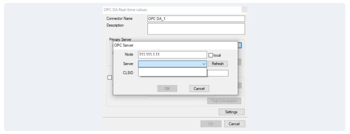
This can be cause by a communication issue between the server and XLReporter. Communication between the OPC server and an OPC client must be verified. If an OPC client is not provided with the server, an independent OPC client is available for download from the SmartSights website.
